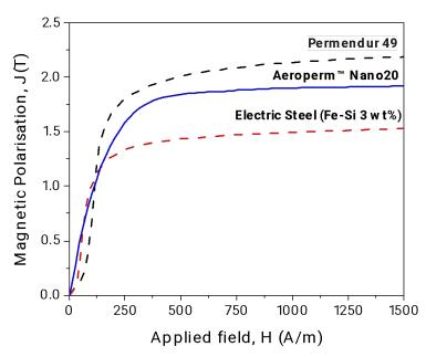
Kite Magnetics Aeroperm™ series of nanocrystalline soft magnetic alloys offer core losses up to one-tenth that of conventional non-oriented 3 wt % iron-silicon steels without sacrificing saturation magnetic polarisation.
